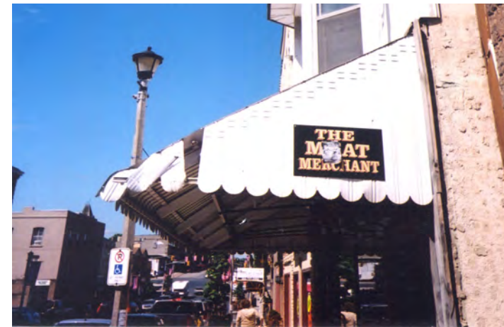
Figure 50 Signage incorporated into awnings should be placed on the side panels and front flaps only. Retractable awnings are preferred over permanent ones.
