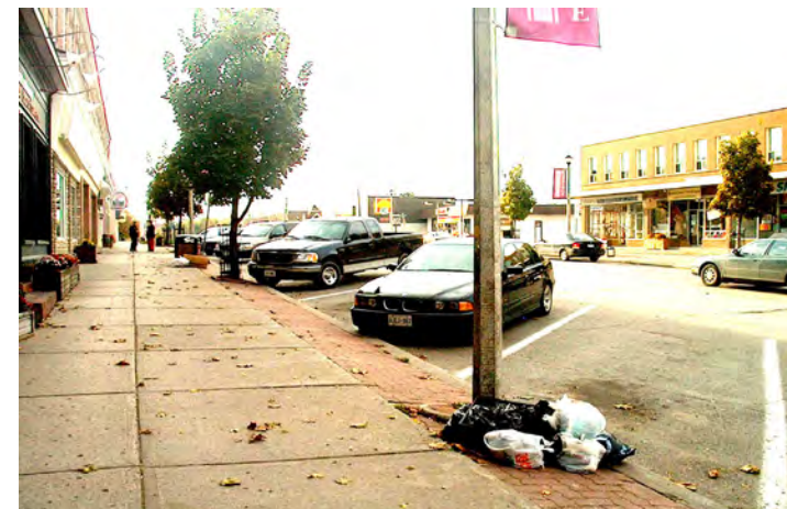
Figure 8 Sidewalks could be widened if angled parking were to be replaced with parallel parking.
