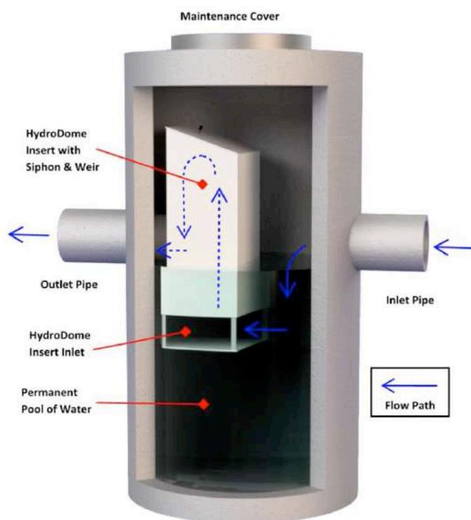
**Figure 1: Schematic of the Hydroworks HydroDome Oil-Grit Separator**
