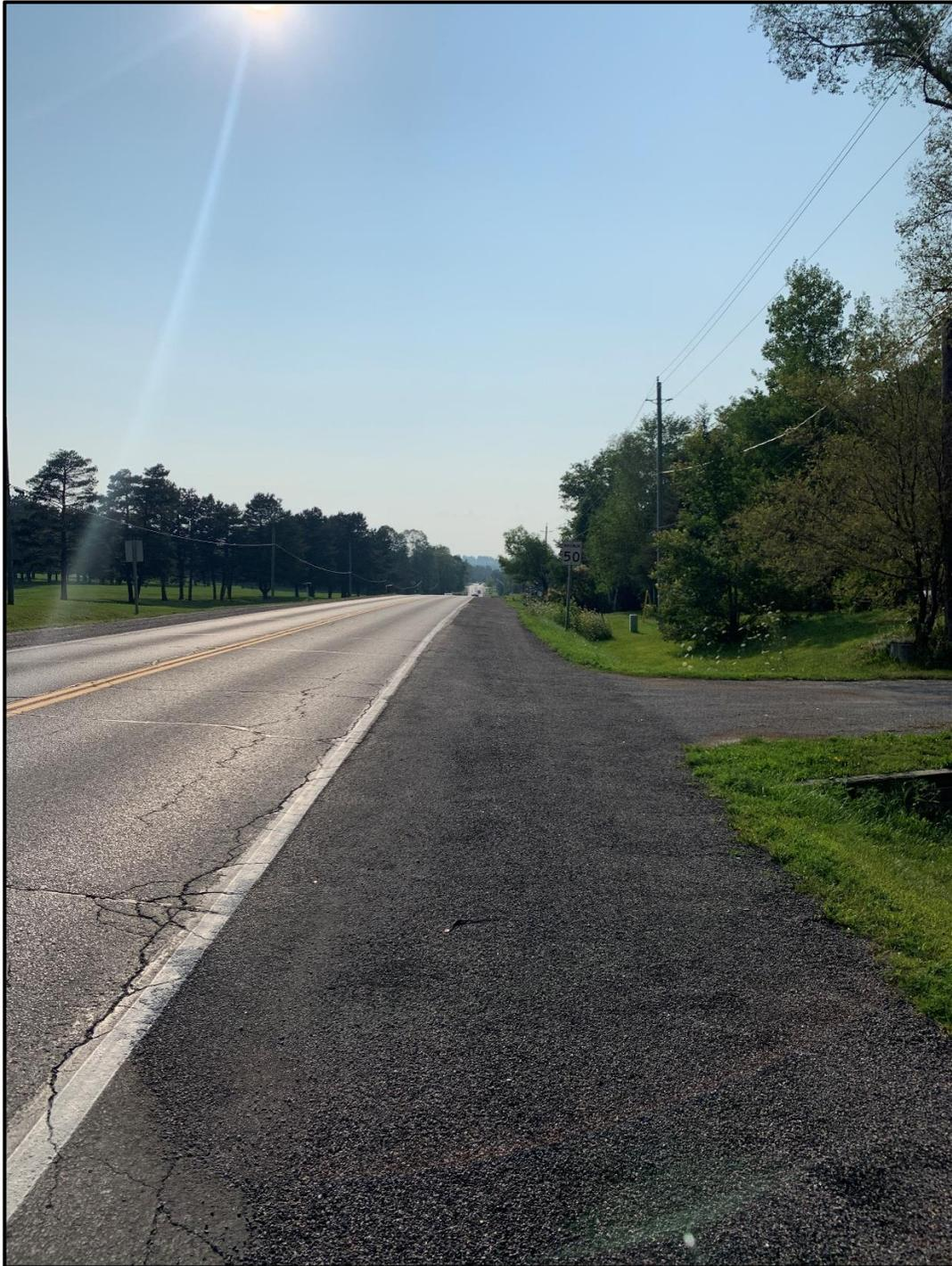
For the purpose of verifying that minimum sight line requirements are met, a design speed of 70 km/hr (posted speed limit plus 20 km/hr) will be utilized for vehicles maneuvering turns from the stop bar onto the major road. Sight distance requirements will be considered for passenger vehicles departing the stopped position at the proposed site accesses on Reach Street.
