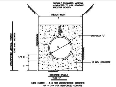
SUITABLE EXCAVATED MATERIAL COMPACTED TO 95% STANDARD PROCTOR DENSITY. TRENCH WIDTH GRANULAR 'C'
