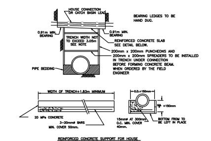
NOTE: WHEN WIDTH OF TRENCH EXCEEDS 3.05m METHOD OF SUPPORTING HOUSE CONNECTIONS AND CATCH BASIN LEADS, WILL BE AS DIRECTED BY THE FIELD ENGINEER.
