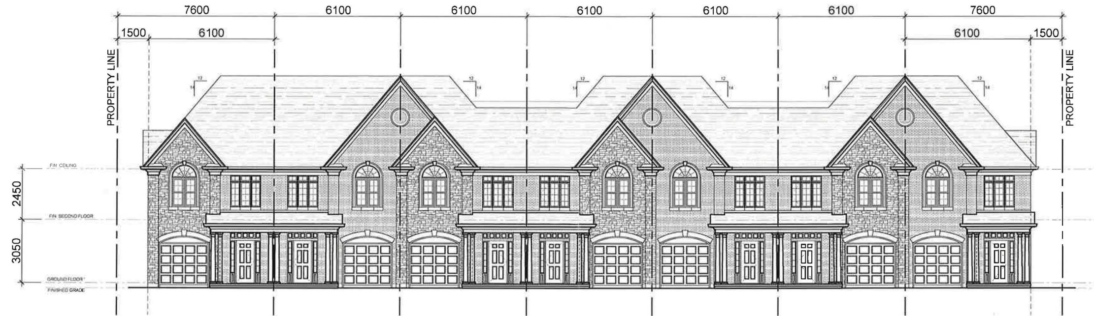
Front Elevation - 7 Unit Block
