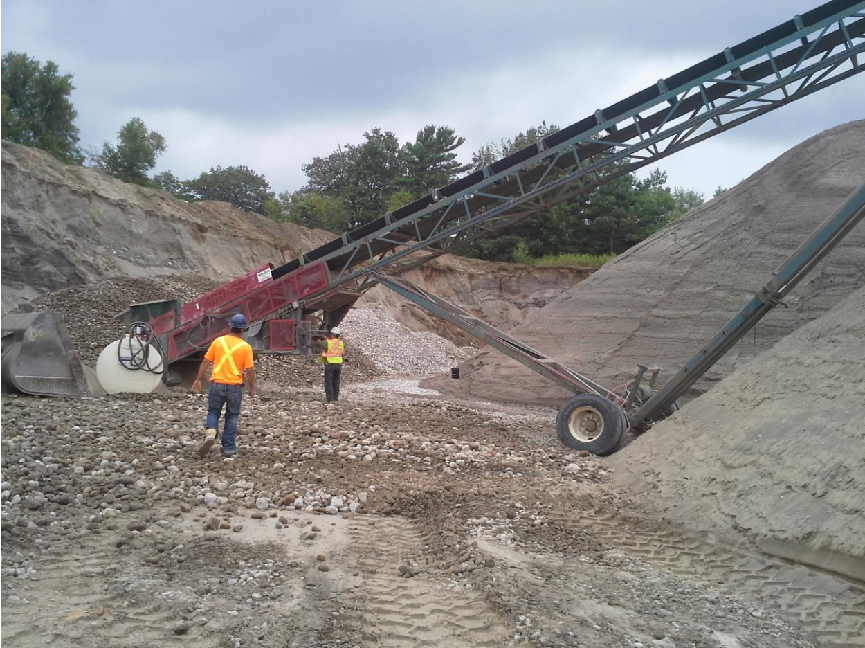
F4: Conveyor/Stacker Unit
