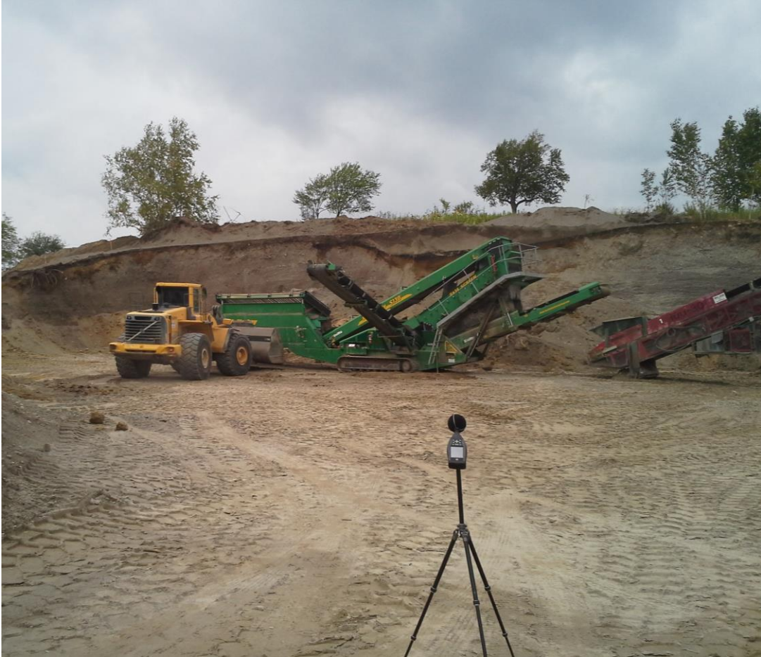
F5: Volvo Front Wheel Loader (Left), McCloskey Screener (Middle), and Conveyor/Stacker Unit (Right)
