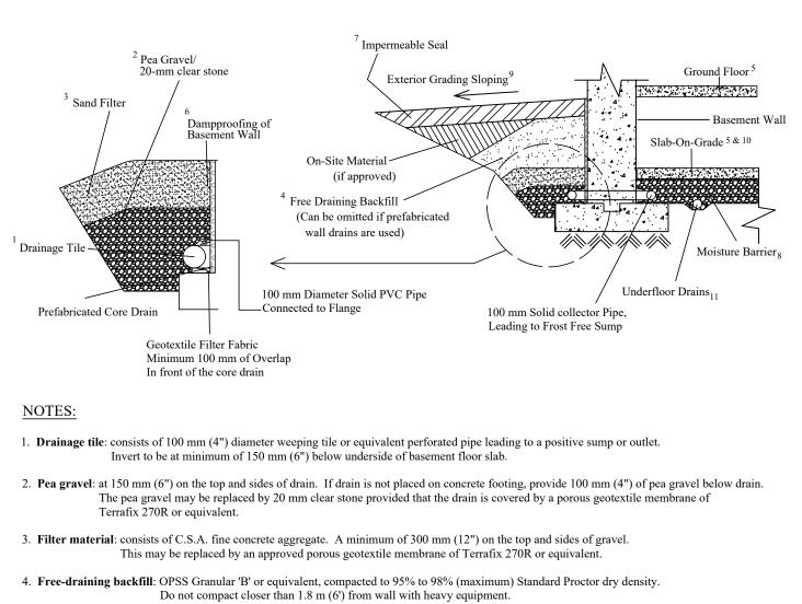
This may be replaced by on-site material if prefabricated wall drains (Miradrain) extending from the finished grade to the bottom of the basement wall are used.
