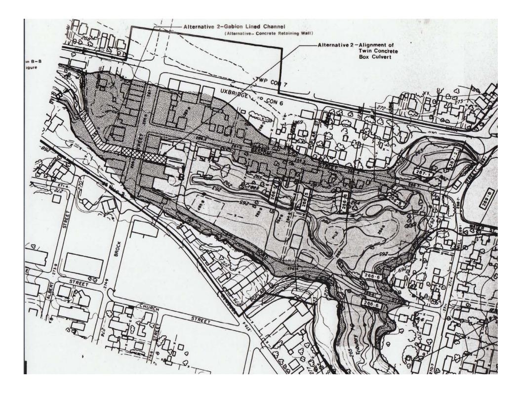
"THE MOST CRITICAL LOCATION FOR FLOOD CONTROL... IS AT BROCK STREET. HERE THE LIMITED FLOW CAPACITY OF THE CULVERT (IN RELATION TO THE REGIONAL STORM) AND THE PRESENCE OF COMMERCIAL STRUCTURES WHICH SPAN THE WIDTH OF THE VALLEY LANDS CREATS A PRECARIOUS FLOOD HAZARD CONDITION."
