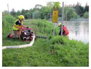
Uxbridge Firefighters Sean Edwards and Doug Noble practice setting up the high-volume portable pump used to refill tankers from static water sources in the rural area.
